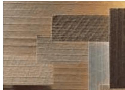
E' COSTITUITA DA CARTA IN PURO KRAFT NORMALIZZATO. I DUE STRATI, CONTENENTI L'ARMATURA, IN FIBRE DI VETRO CON TRAMA ROMBOIDALE, SONO ACCOPPIATI CON SISTEMA HOT MELT.
